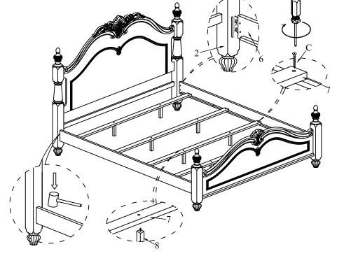
Tool required: Open end wrench and allen key (Included). Philips crew drive (Not included)
